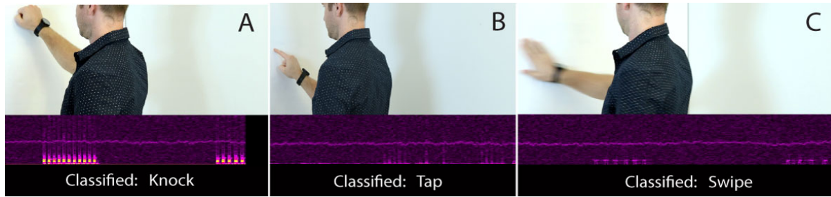
Fig. 9. A variety of surface gestures such as a knock (A), tap (B) and swipe (C) can be reliably detected in discrete locations as seen in their respective spectrograms.
